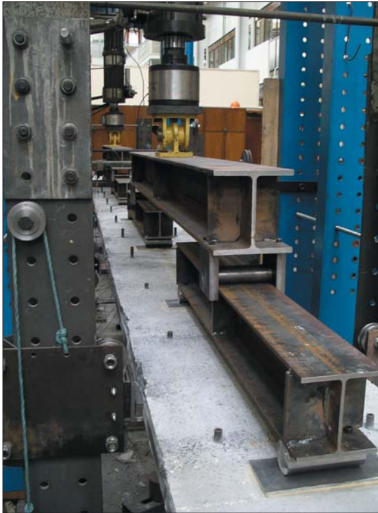
Fig 14. (left) Loading tree for cyclic and ultimate loading
