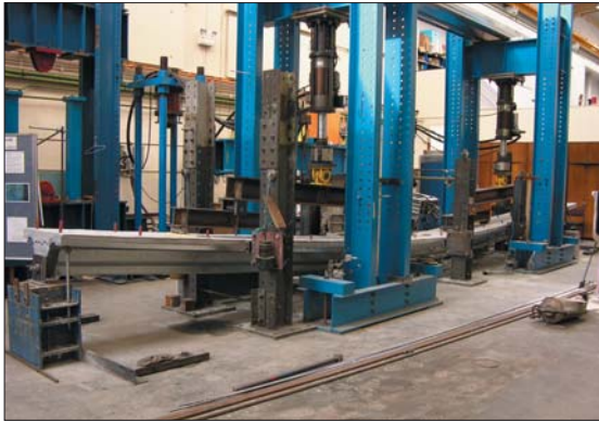
Fig 18. (left) Deck tested to maximum displacement capacity of jacks.
