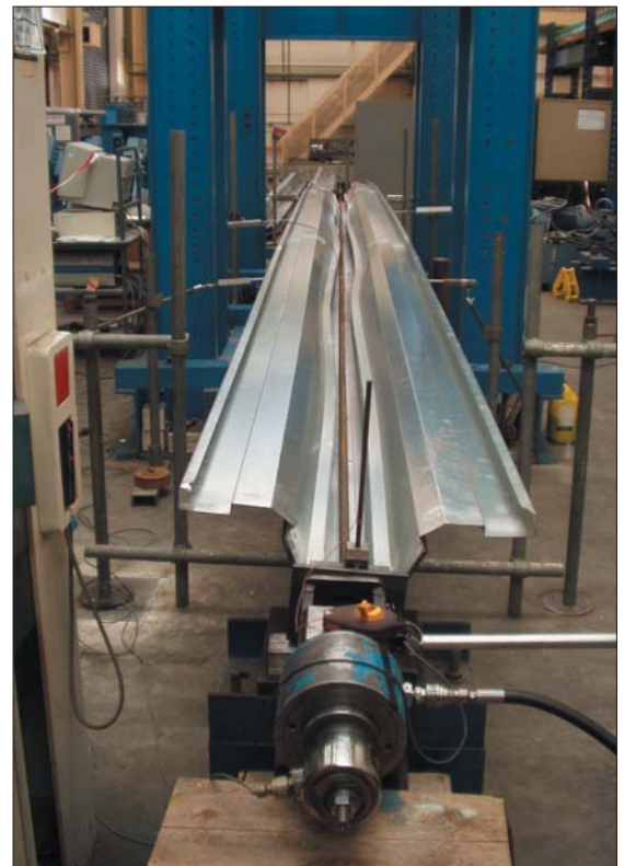
Fig 5. Failure of deck under prestressed load
