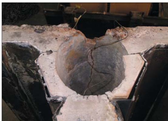
Fig 21. (above) Recorded temperatures through the deck Fig 22. (left) Picture of composite deck following the fire test (note the debonding of the deck)
