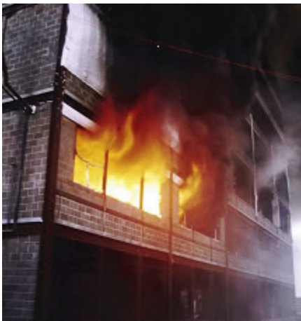
Figure 1 – Fire test on the Cardington steel building (Test 6)
