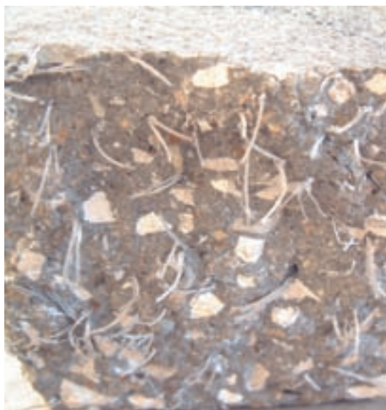
Polypropylene fibres provide protection against spalling.
