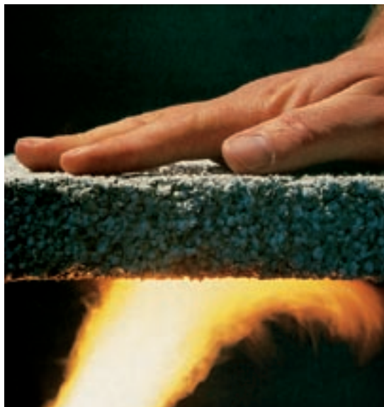
Concrete provides protection against heat from fire.
