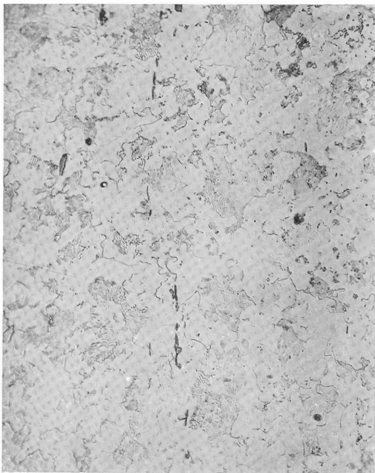
MILD STEEL REINFORCING BAR AS RECEIVED. ( \times 500 .)
