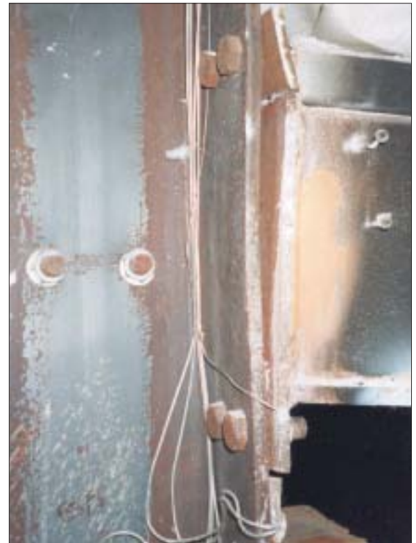
Fig 9. (Above) Photographs showing fracture of plate (end-plate) and shear failure of bolts (fin plate)
