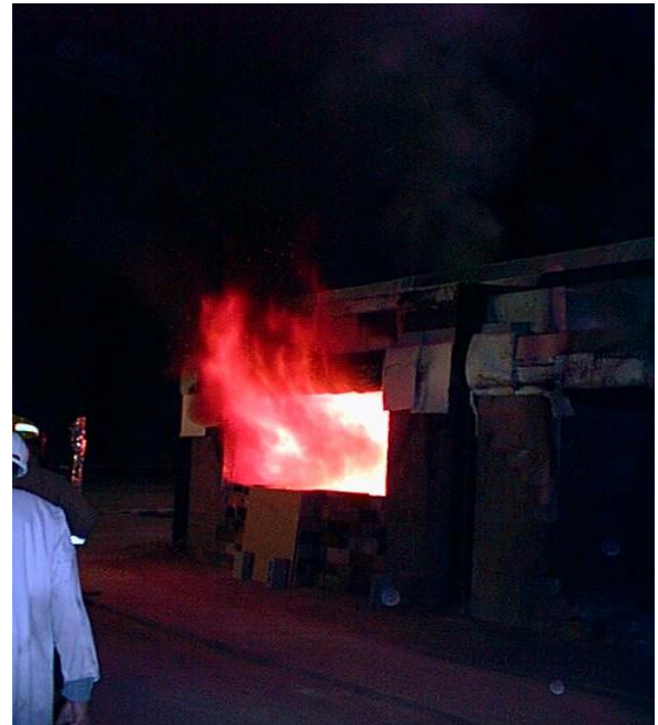
Figure 23 Slab B post-flashover
