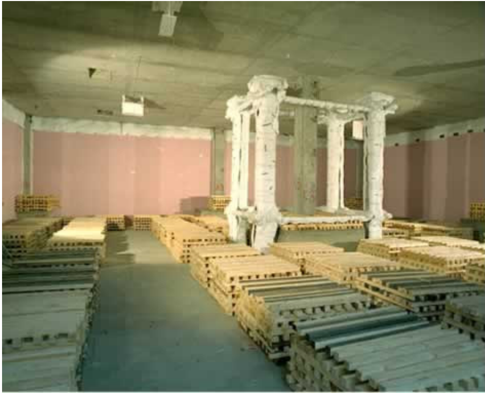
Figure 4 Fire compartment prior to ignition (looking from the openings along gridline D)
